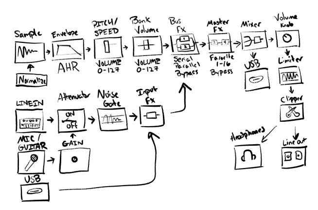
Even for the rather simple architectural design of the mk2, there is a \*lot\* going on here to take in, and many things that can impact the volume from sample or input, all the way to your outputs on USB, Headphones, or Line Outputs.
