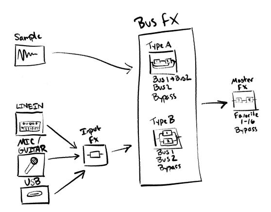
As of firmware 2.0, Roland has added a setting to determine if your samples that are skipping the Bus FX section should go to the Master FX or if they should bypass the Master FX. This
